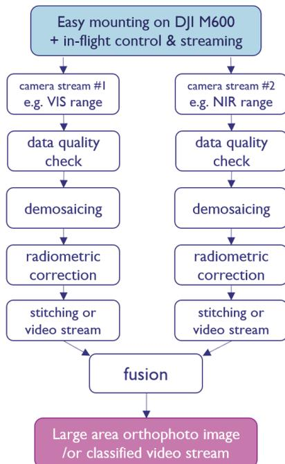
Software processing pipeline (high level overview) starting with RAW frame acquisitions from two hyperspectral imaging sensors (e.g. VIS + NIR) to fully stitched orthophoto images.
